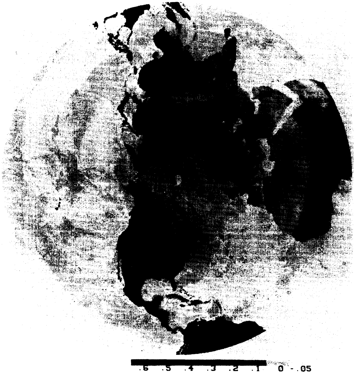
Figure 9.- Northern Hemisphere composite AVHRR image of the normalized difference vegetation index [(\text{channel } 2 - \text{channel } 1)/\text{channel } 2 + \text{channel } 1] for August 23-29, 1982.
