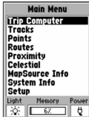
Step 4: Using the **ROCKER** key, rocker down to the Setup option and press the **ENTER** key. The screen shown below should now appear.
