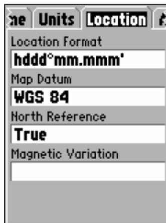
Step 6: Using the **ROCKER** key, rocker down once to the Location format and press the **ENTER** key.
