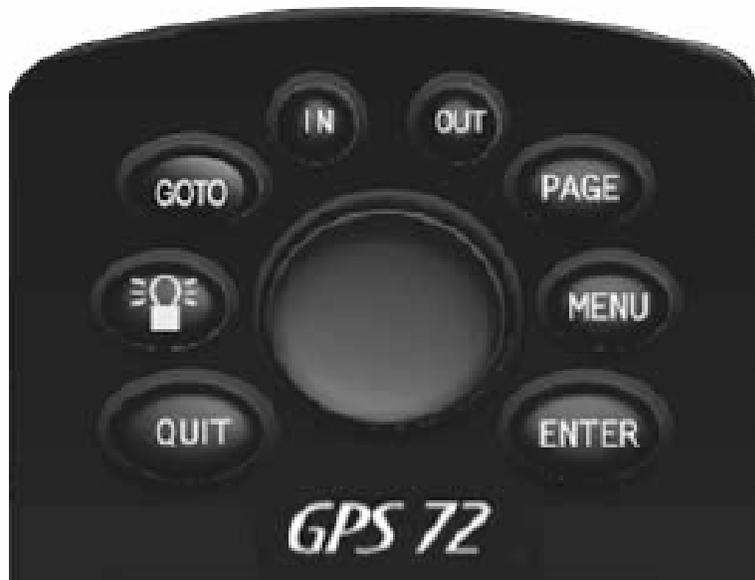
**POWER** Used to turn the unit on and off. To turn the unit off, press the POWER key and hold it. The POWER key is also used to display the adjustment window for the back light and contrast. To activate the back light/contrast adjustment window, press and release the POWER key.
