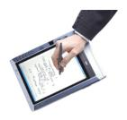
A second way to enter information is to use a keyboard that appears as part of the screen. This on-screen keyboard is operated with the tablet's pen.
