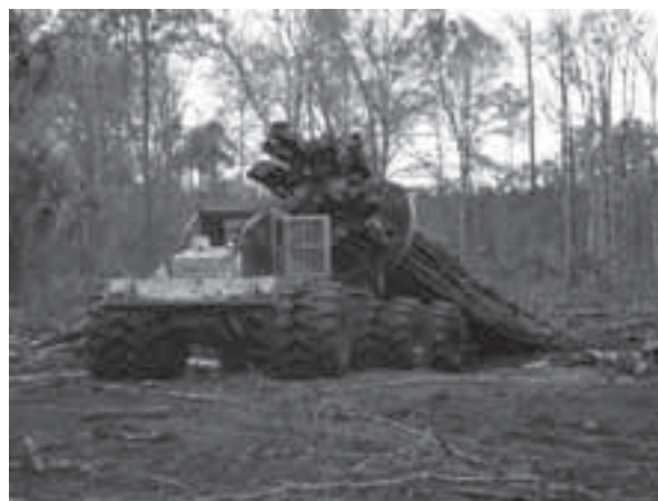
A skidder bundles roundwood from a timber harvest to be loaded on semis.
